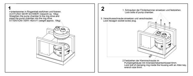
Pay attention to the following torque values: Image 2 item 1: Bolts pump chamber 28 Nm (20.7 lb-ft) Image 2 item 2: Bolt clamping ring 8 Nm (5.9 lb-ft)
