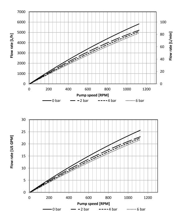
The flow rates showing at the chart above were ascertained with new diaphragms and new valves under standard conditions after the final assembly of the pump.
