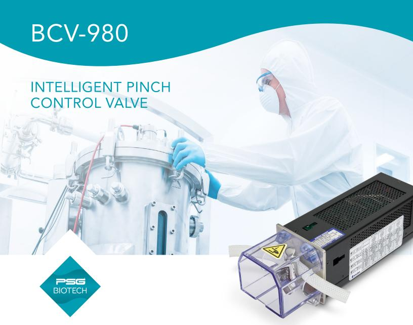
The BCV-980 is a compact, cost-effective, high-performance pinch control valve designed for biotechnology and pharmaceutical industries. The intelligent control valves utilize PSG Biotech's proprietary integral PID control algorithms. The valve monitors up to four analog signals from external sensors or controllers and modulates the valve position accordingly.
