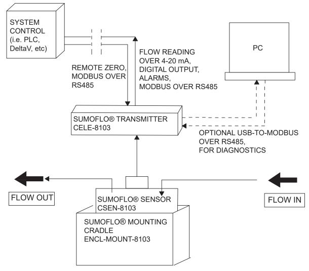
An ultra-low flow SumoFlo<sup>®</sup> CPFM-8103-series Coriolis flow meter consists of three components: the singleuse Coriolis flow sensor, the durable transmitter, and the durable mounting cradle, as well as the durable cables to connect the transmitter to the sensor and the transmitter to the system control device. When properly installed in the mounting cradle, the SumoFlo<sup>®</sup> flow meter meets CE specifications.
